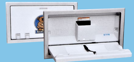
KB100-ST HORIZONTAL, RECESSED-MOUNTED WITH STAINLESS STEEL FLANGE Dimensions: 37" W × 23" H (940 × 584mm). Depth (closed): 1/2" (6.35mm). Extension (open): 15" (381mm) from flange. Rough Wall Opening: 35 1 / 2 " W × 20 1 / 2 " H (900 × 529mm). Depth: 4 1 / 4 " min. (102mm). Colors: Cream, Grey, White Granite. Material: 18-gauge type 304 satin-finish stainless steel with polyethylene
