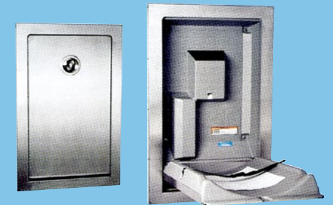
KB111-SSRE VERTICAL, SEMI-RECESSED MOUNTED Dimensions: 24 1 / 4 " W × 39 1 / 2 " H (616 × 1003mm). Depth (closed): 5 1 / 2 " (38mm). Extension (open): 20 1 / 2 " (793.75mm). Rough Wall Opening: 22 1 / 8 " W × 35 5 / 8 " H (562 × 905mm). Depth: 4" min (102mm)
