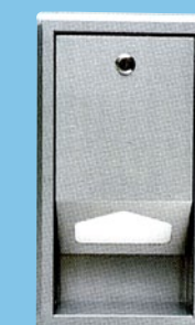
KB100-ST HORIZONTAL, RECESSED-MOUNTED WITH STAINLESS STEEL FLANGE Dimensions: 37" W × 23" H (940 × 584mm). Depth (closed): 1/2" (6.35mm). Extension (open): 15" (381mm) from flange. Rough Wall Opening: 35 1 / 2 " W × 20 1 / 2 " H (900 × 529mm). Depth: 4 1 / 4 " min. (102mm). Colors: Cream, Grey, White Granite. Material: 18-gauge type 304 satin-finish stainless steel with polyethylene
