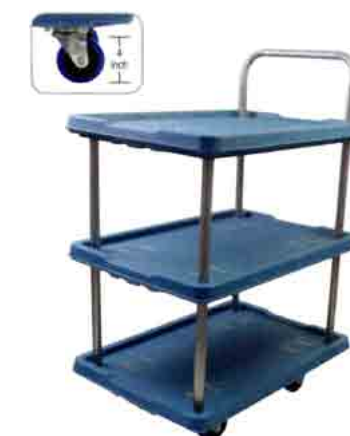
287-R Three layer Platform Trolley Specification:780L × 540W(mm) Unfold dimension:780L × 540W × 1,105H(mm) Wheel Size:4 inch Layer Distance:300 mm Total Loading:100 kg
